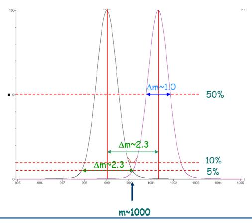
❖ The numerical value arrived at using the FWHM definition is always larger than the value one would determine using the 10% valley definition.
