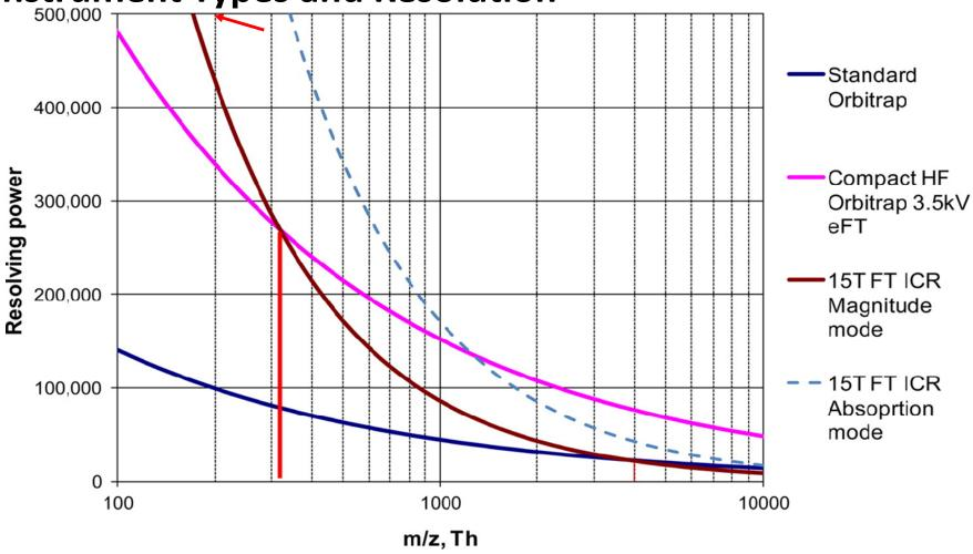
Dependence of resolving power on m/z for the following analyzers (all data are shown for a 0.76 s scan): (i) standard trap (magnitude mode, 3.5 kV on central electrode), (ii) compact high-field trap (eFT, 3.5 kV on central electrode), (iii) FTICR (magnitude mode, 15 T), (iv) FTICR (absorption mode, 15 T).
