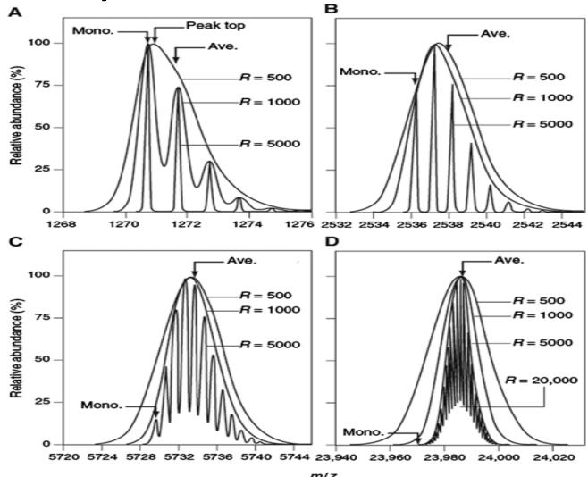
Good mass accuracy can only be obtained from sufficiently sharply and evenly shaped signals.
