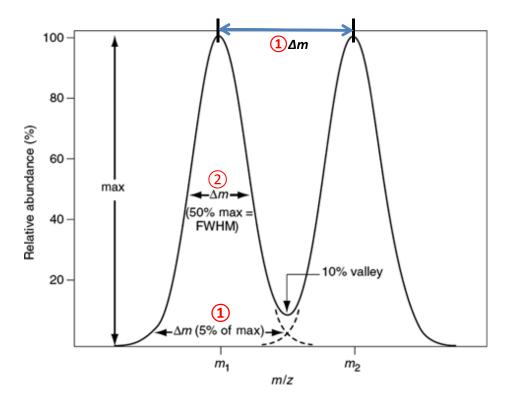
10% valley conditions are fulfilled if the peak width at 5% relative height equals the mass difference of the corresponding ions. (5% + 5% = 10%)
