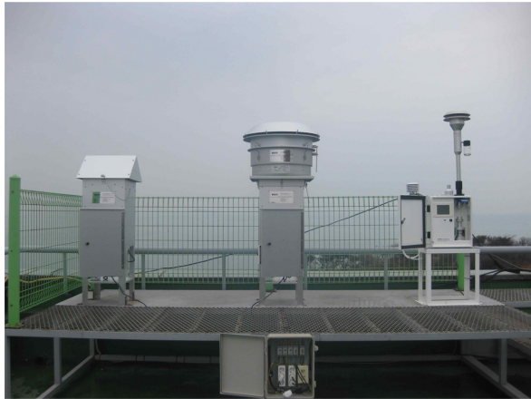
Fig. 3. Air pollution monitoring equipment as a sample collector of the Asian dust for the weekly iron profile.
